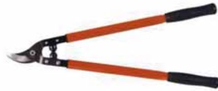
P-2275 P16-60 P-2273 P16-40 Lopping shear with fully hardened and stamped steel cutting blade and forged counter blade mounted with shear pin to avoid damage to cutting edge. Bypass cutting action, Length: P16-60 60cm, P16-40 40cm.
