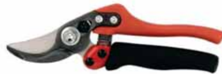
P-1120 P2-22 Ideal professional secateur for heavy duty use. Modern lightweight carbon and glass fibre handles which rotate to reduce effort, prevent fatigue and increase user comfort. Stamped blades and counter blade with sap groove. P2-22 cutting cap. of 25mm. Length: 22cm.
